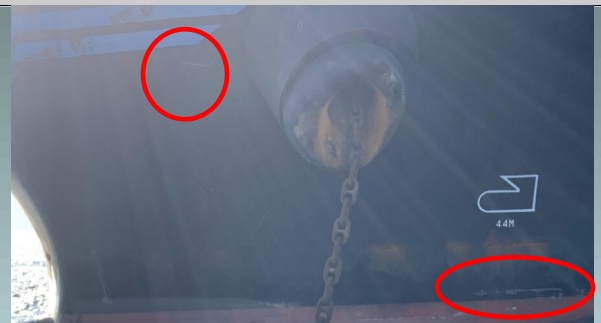
Figure 2: The paint scratches on the port bow of EPHESOS
