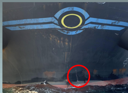
Figure 1: The paint scratches on the stem of EPHESOS
